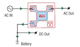
The total output power of a module can be shared between the AC load, DC load and charging power based upon the requirement.
