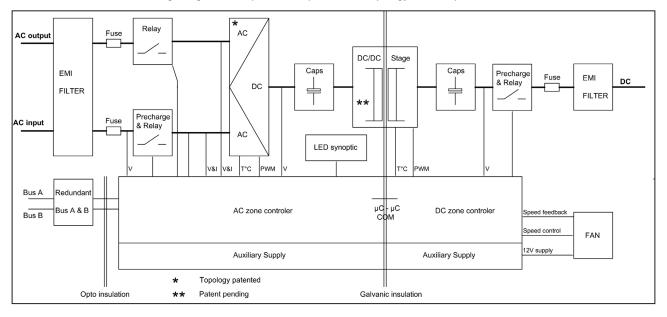
The below block diagram gives an explicit description of the topology and its operation.
