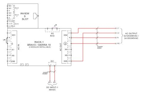
1\* -----> REG\_MODE [MEN] CONNECTION B/W AC OUTPUT NEUTRAL AND EARTH 3\* -----> TO BE REMOVED WHEN EXTERNAL REMOTE USED
