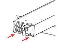
Push firmly until module is engaged
