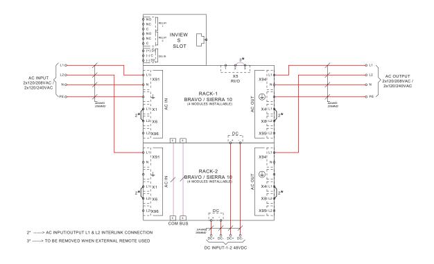
Split phase - Wiring diagram
