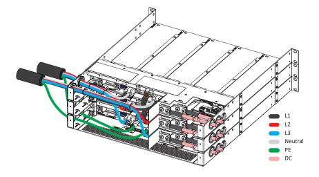
Three phase - Cable connections
